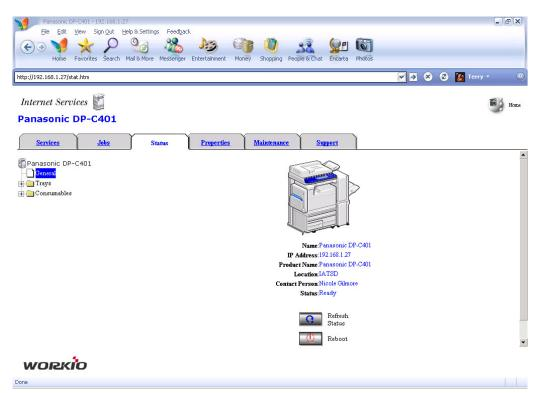
**Figure 5** – The Panasonic WORKiO DP-C401's *Internet Services*' printer Web page. *Internet Services* enables users to view the DP-C401's status and availability via a standard Web browser, and does not require the installation of any software on the user's workstation. Administrators may also remotely monitor and configure network settings with *Internet Services*.
